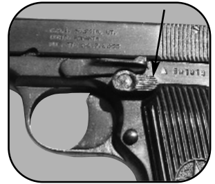
Safety lever in the horizontal or “SAFE” position (covering dimple/stamped dot on receiver).
